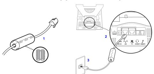
The following figure shows how to connect the phone to the network.
